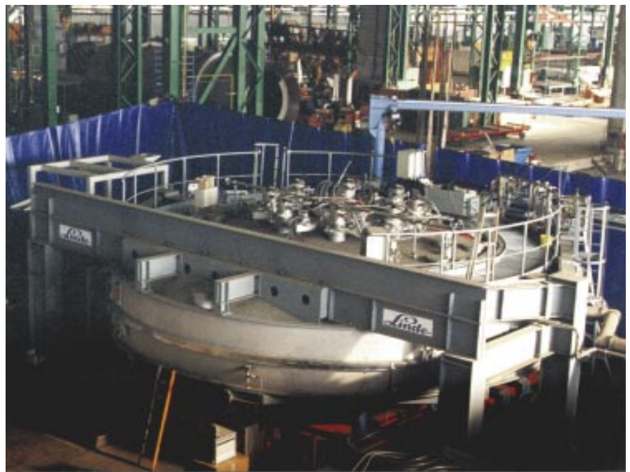
Figure 1: The coating unit for the VLT mirror substrates at Deggendorfer Werft premises. The circular platform on top of the chamber provides personal access to the cryo-pumps, feedthrough, vacuum gauges, etc. located on top of the chamber.
