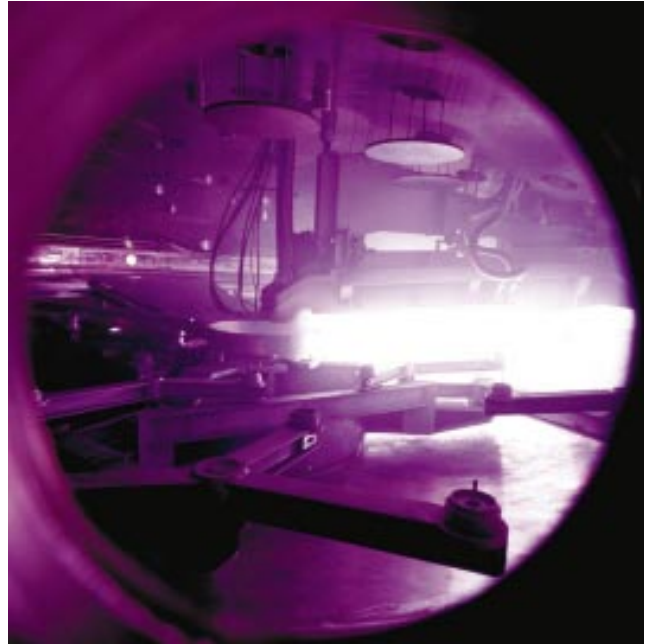
Figure 3: A view through one of the vacuum chamber windows while the glow discharge cleaning device is fired. The blue light is emitted from the plasma generated by the glow discharge electrodes. Above the shiny discharge area the contours of the sputter source arrangement are visible. In the lower part of the picture one recognises the whiffle-tree loaded with the dummy.
