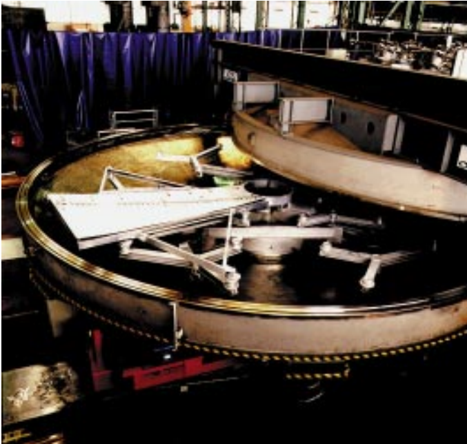
Figure 2: The lower part of the coating unit vacuum chamber moved out beneath the fixed upper part. Inside the chamber the rotatable whiffle-tree for support of the primary mirror is visible. Here, a steel plate serves as a dummy mirror for testing purposes.
