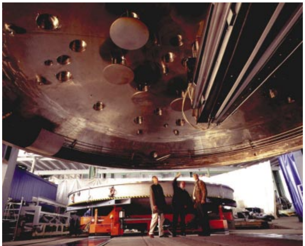
Figure 4: The 'giant dome' – The upper vacuum chamber part carrying the sputter source arrangement (top right) and the catcher disks below the cryo-pumps (top centre). The lower chamber part is transported out by means of the air cushion cart (orange) moving along the metallic strips (bottom left and right).
