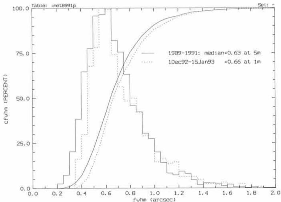
Figure 2: Statistics of seeing measurements before and after summit levelling. Seeing is computed for equivalent 20-min exposures obtained at  $0.5 \mu\text{m}$  at zenith with a perfect large telescope.
