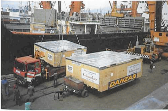
Figure 2: Loading of the NTT boxes onto the ship in Genova harbour, 29 April 1988. In the front of the picture the box containing the base of the fork is visible. This box weighs about 44 tons.
