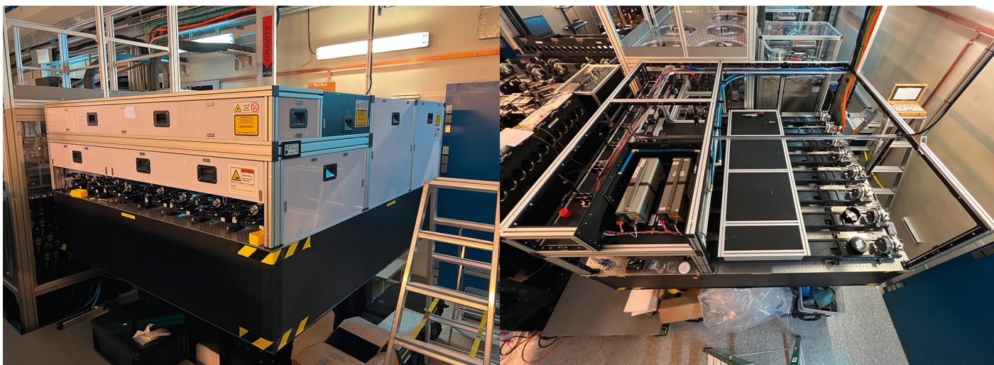
Figure 2. The left panel shows the enclosure of the beam compressor delay line optical bench; the right panel shows a bird's-eye view with the protective panels removed. The eight newly activated beam compressors can be seen towards the right of the images; they stretch, however, the entire length of the bench. The two grey laser heads on the top feed the laser distance metrology system that monitors the optical path length to better than 2 nm precision at all times.
