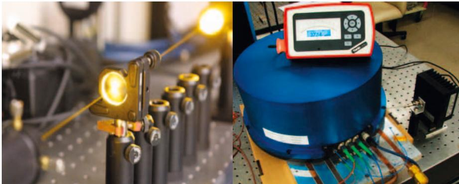
Figure 7. Left: The ESO Raman fibre laser used to test laser optics coatings for the launch telescope. Right: The single arm Raman fibre amplifier from MPB/TOPTICA showing the required 37.4 W of infrared 1178 nm power for the proper Na wavelength output power (image from April 2010).
