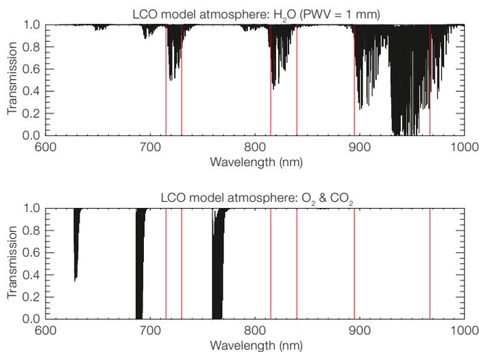
Figure 1. Atmospheric transmission in the optical to near-IR domain. Upper panel: absorption caused by 1 mm of H<sub>2</sub>O. Lower panel: absorption resulting from O<sub>2</sub> and CO<sub>2</sub>. The analysis described uses wavelength regions (denoted in red) in which absorption is from water vapour only, allowing the atmospheric content of PWV to be derived. This wavelength range was chosen for the analysis of the archival data, but suitable windows exist over a very wide wavelength extent.
