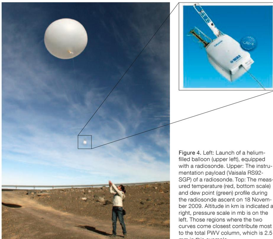
Figure 4. Left: Launch of a helium-filled balloon (upper left), equipped with a radiosonde. Upper: The instrumentation payload (Vaisala RS92-SGP) of a radiosonde. Top: The measured temperature (red, bottom scale) and dew point (green) profile during the radiosonde ascent on 18 November 2009. Altitude in km is indicated at right, pressure scale in mb is on the left. Those regions where the two curves come closest contribute most to the total PWV column, which is 2.5 mm in this example.
