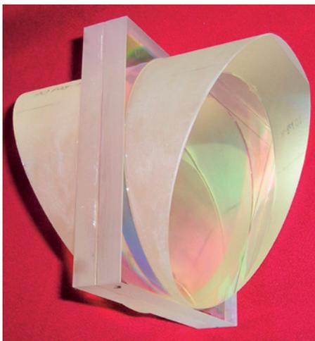
Figure 2: The VPH grism as hosted inside the new mounting.
