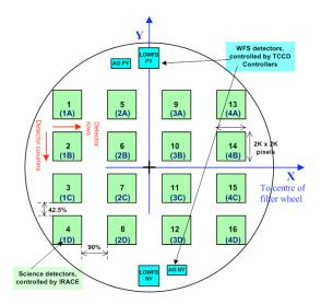
Figure 8: VIRCAM focal plane geometry
