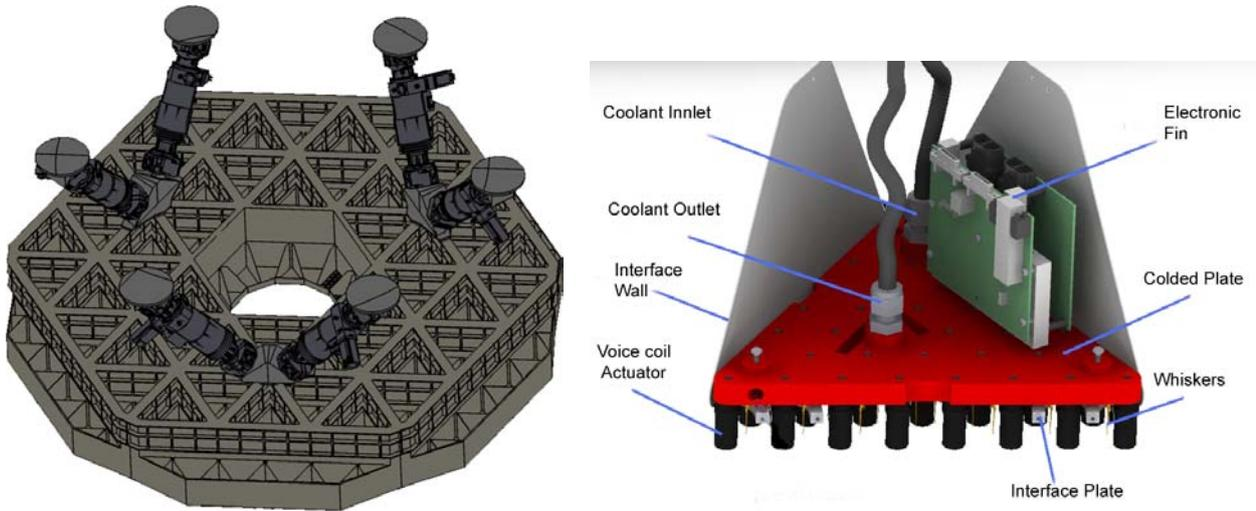
Figure 3: Left: reference body structure. It is the reference surface for the thin mirror shell. It need optical surface quality in term of flatness and must be stable with gravity and temperature. Right: Bricks: mechanical structure supporting ~30 actuators, the associated electronics and used to cool down the system.
