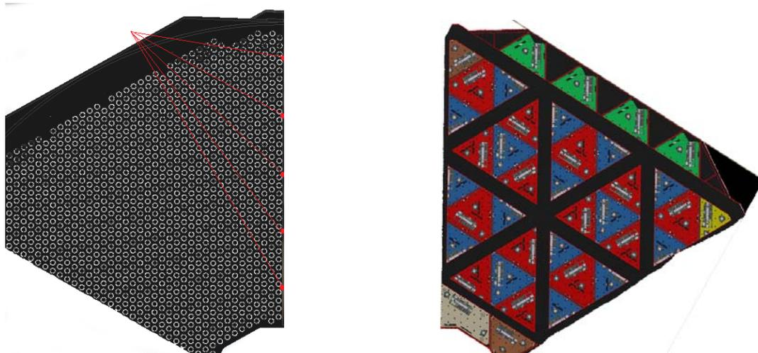
Figure 4: Sixth of the reference body seen from the front side: all the actuators holes are visible. Sixth of the reference body seen from the back side: the triangular structure of the reference body as well as the bricks is visible.
