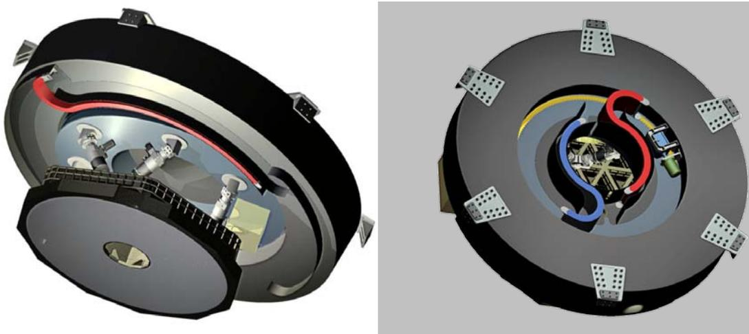
Figure 2: M4 Baseline design. The M4 Mirror is visible on the left figure as well as the hexapods while the cable wrap and fixation interface to the telescope is visible on the right figure.
