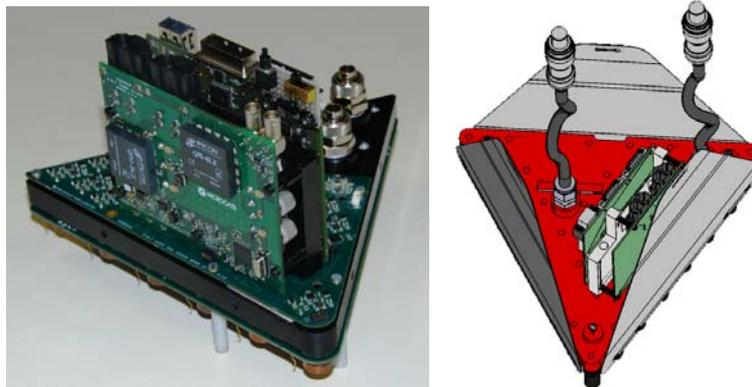
Figure 5: Left: First brick prototype designed in the frame of the previous contract. The extensive test of the Demonstration Prototype allowed Microgate and A.D.S. International to improve to design in term of mounting on the reference body, improving as well the cooling and updating the electronics design. Right: Baseline brick design. The three material plates allow a better alignment of the brick in the reference body structure and make the maintenance easier.
