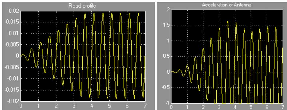
Figure 3 Transporter Response without additional damping system.
