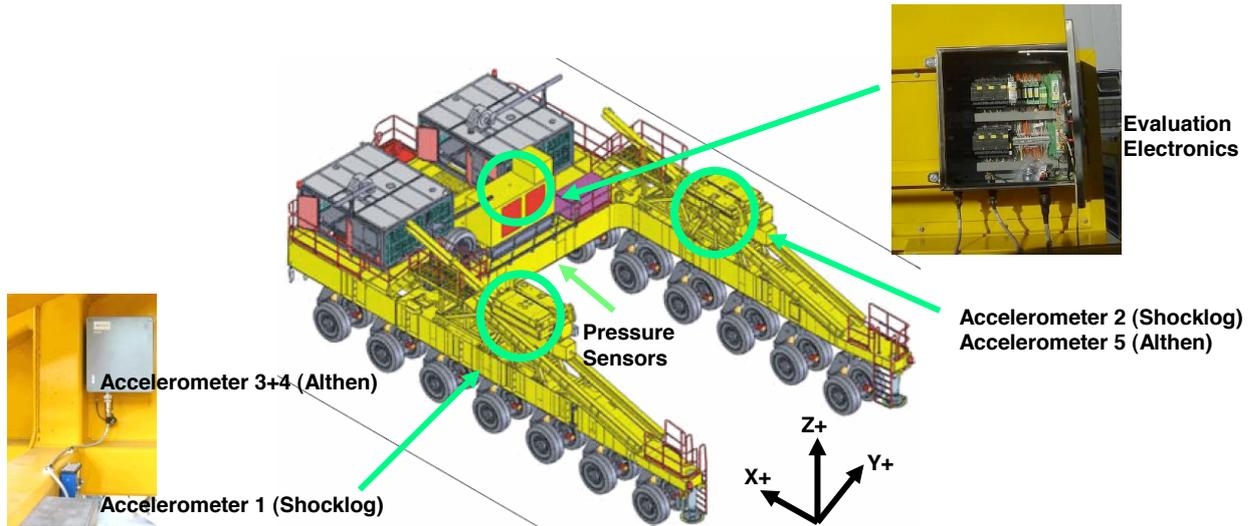
Figure 9 Main components of the Automatic Stopping System
