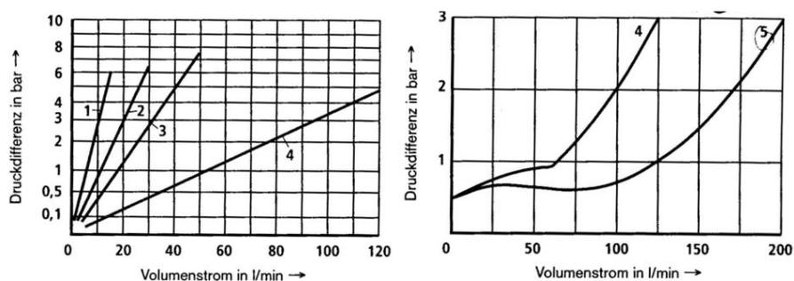
Figure 6 TCV Characteristics from Bosch Rexroth (size 4 was chosen, left throttle, right check valve)
