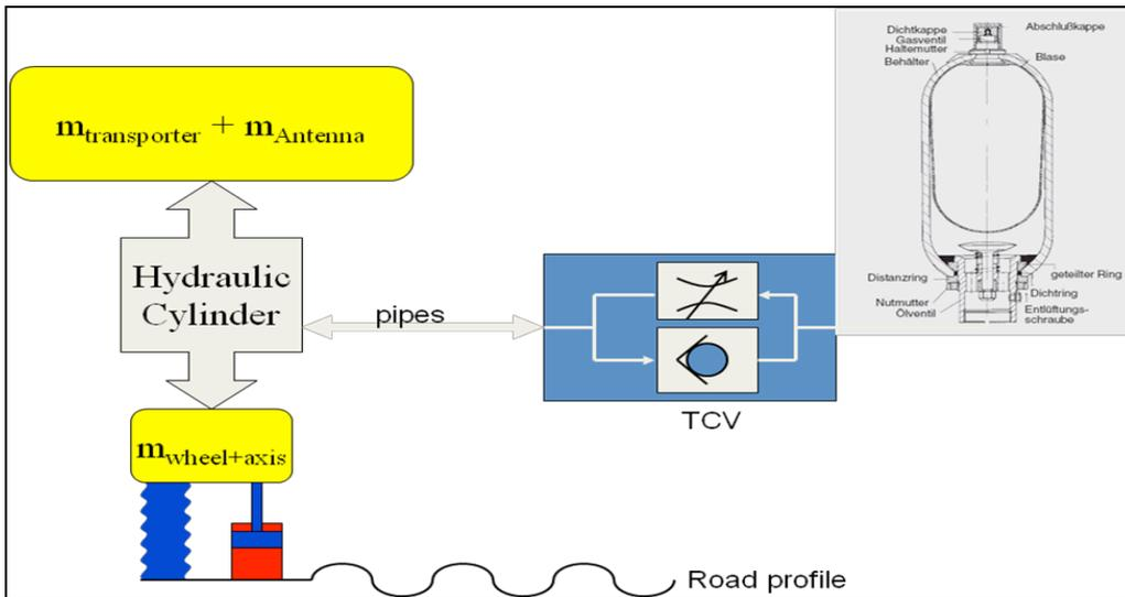
Figure 4 Working principle of the damping system (accumulators [5] and throttle-check valves [6] are added to the transporter)
