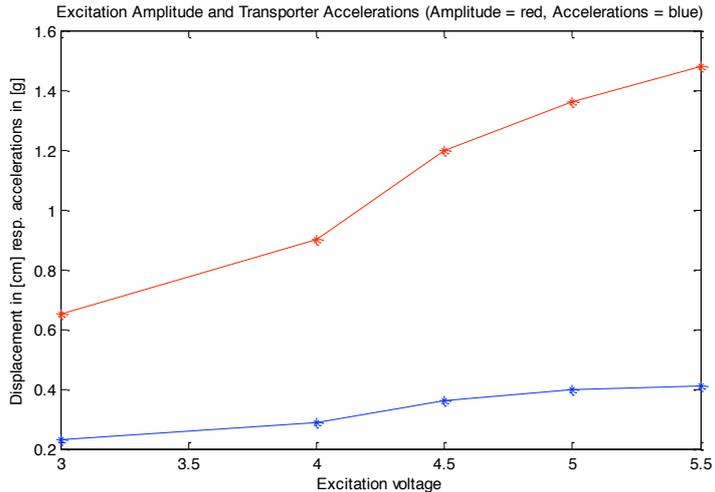
Figure 12 Wheel Cylinder Displacement and Acceleration of Transporter #1 (Otto) as a Function of Excitation Amplitude (Saturation due to Damping System)
