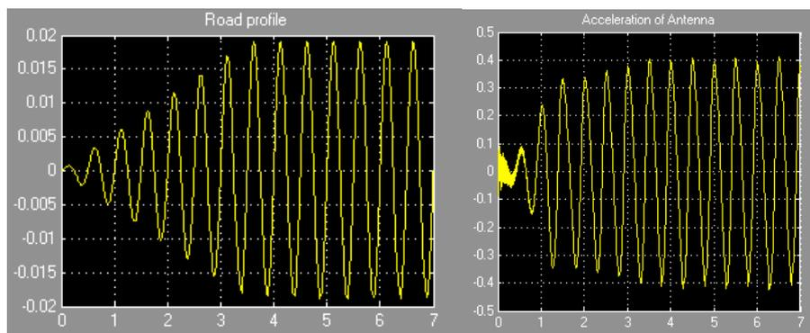
Figure 7 Transporter Response with additional damping system.
