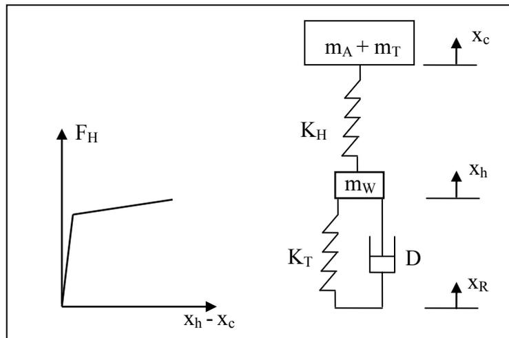
Figure 5 Simplified mechanical model (releasing oil into accumulators changes  $K_H$ )
