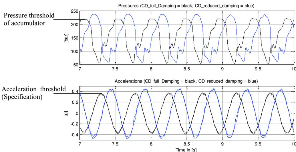
Figure 11 Increase of hydraulic pressures due to partial disable of accumulators, Black = All on, Blue = Some off
