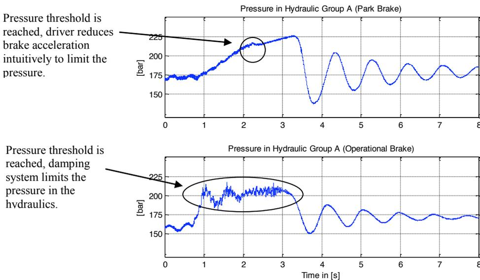
Figure 13 Pressure and Acceleration History during Transporter Brake Test (note: the pressures are measured a few meters away from the running gears, therefore quasi-static pressure changes seem to be higher than fast ones)
