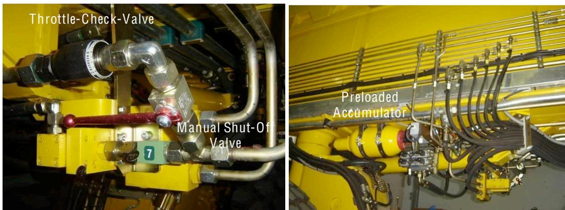
Figure 8 Additional hydraulic components at each wheel pair
