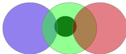
In this example, the centering is performed in the green, some light is lost due to the size of the pinhole with respect to the PSF. The light coming from the blue and red wavelength is also strongly lost. However because the objects adapted of this mode are extremely bright this is not so an issue.
