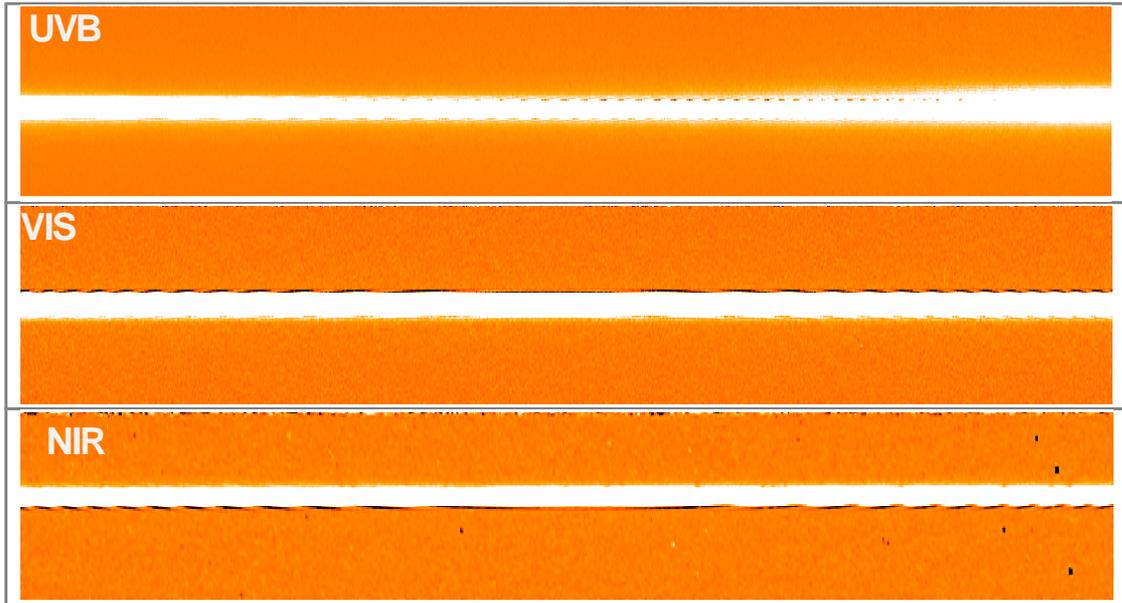
**Figure 1:** Cutouts of the final 2D spectrum for Achernar ( $V = 1.1$ ,  $K = -4.1$ ). The top panel shows the UVB arm from 435 – 450 nm, the middle panel shows the VIS arm from 770 – 785 nm, and the bottom panel shows the NIR arm from 1720 – 1755 nm. In the VIS and UVB arm, the wiggles are visible in the top edge of the trace. In the NIR arm, the wiggles are visible in the lower edge of the trace.
