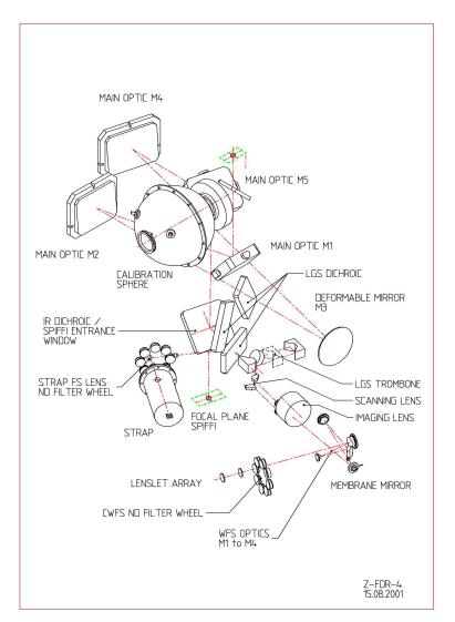
Figure 13: Optical layout of the AO module
