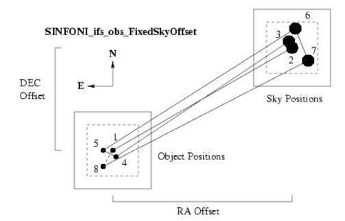
Figure 24: An illustration of the offset sequence taken with the FixedSkyOffset template. ("Number of exposure per Offset" = 1). The large circles for the sky position indicate that these observations are performed in open loop.
