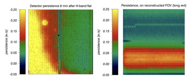
Figure 3: The left image shows a map of detector persistence pattern. The right image is a reconstructed SPIFFI image, showing how the persistence varies over the FOV of the instrument. The bottom of the FOV is made up of pixels from the left side of the detector (where persistence is high), and the top of the FOV is made up of pixels from the right side of the detector (where persistence is low).
