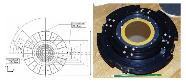
Figure 15: DM electrode geometry – DM/TTM assembly
