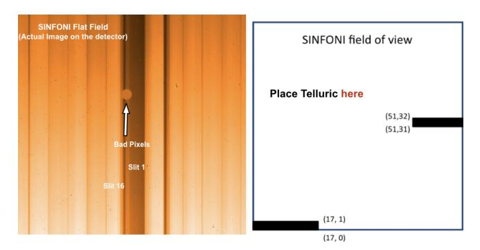
Figure 9: *Left:* This is a SINFONI Flat Field image. The disc of bad pixels near the centre of the detector mostly falls on slit #1, which crosses the centre of the field of view of SINFONI. *Right*: This is the reconstructed FOV of SINFONI, showing the location of the blind spots. Slit #16 corresponds to y=31 and 32. Slit #1 corresponds to y=0 and 1.
