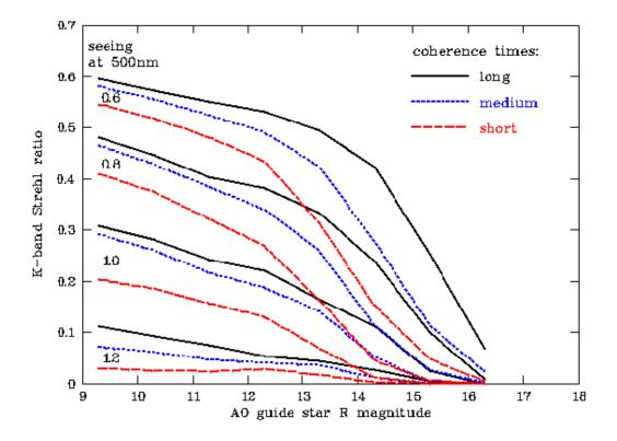
Figure 17: NGS performance for a wide range of optical seeing values (0.6 to  $1.2^{\prime\prime}$  ) and long, medium and short coherence times.
