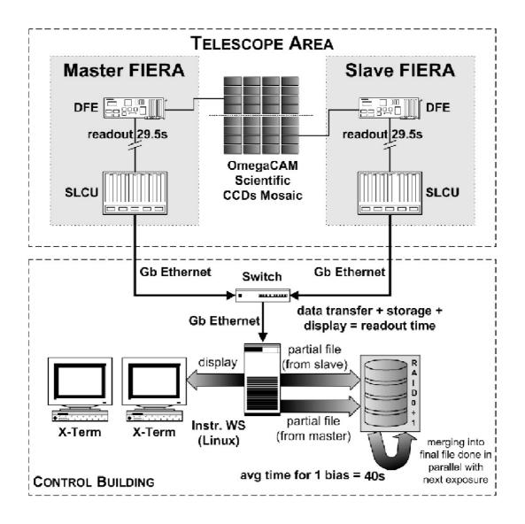
Figure 7: Data flow diagram for readout of the OmegaCAM science array.
