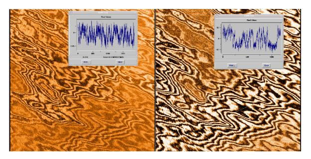
Figure 30: excerpts of a fringe map for the Sloan i' (left) and z' band (right). Intensity contrasts in the image are at  $\pm 5\%$ . The cuts show that fringe amplitudes are a few percent in i', and up to 10% in z'.
