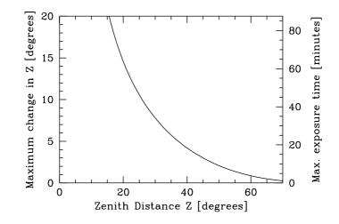
Figure 23: The maximum change  $\Delta Z$  in zenith distance (degrees) that is allowed during an exposure before the image quality is degraded by 0.1 arcsec due to atmospheric refraction. The right-hand axis approximately translates this limit into an exposure time T (minutes) for a field on the equator, as seen from the Paranal latitude of  $-24^{\circ}$ :  $T = 4\Delta Z/\cos(-24^{\circ})$ .
