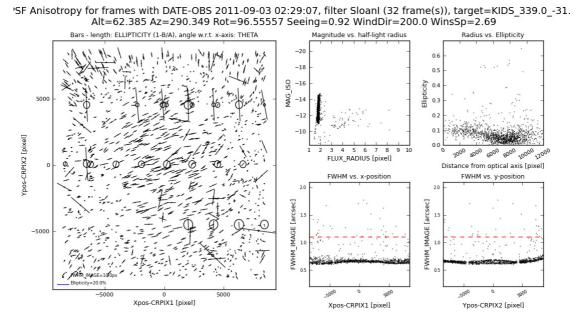
Figure 24: PSF anisotropy analysis plot obtained for an i-band observation. For the given example, outside seeing as indicated by the DIMM (around V-band) was 0.9'', and IQ on OmegaCAM chips was ~0.65''. In general, IQ variations of 10-25% across the FOV can occur, depending on outside seeing, filter and telescope mirror position.
