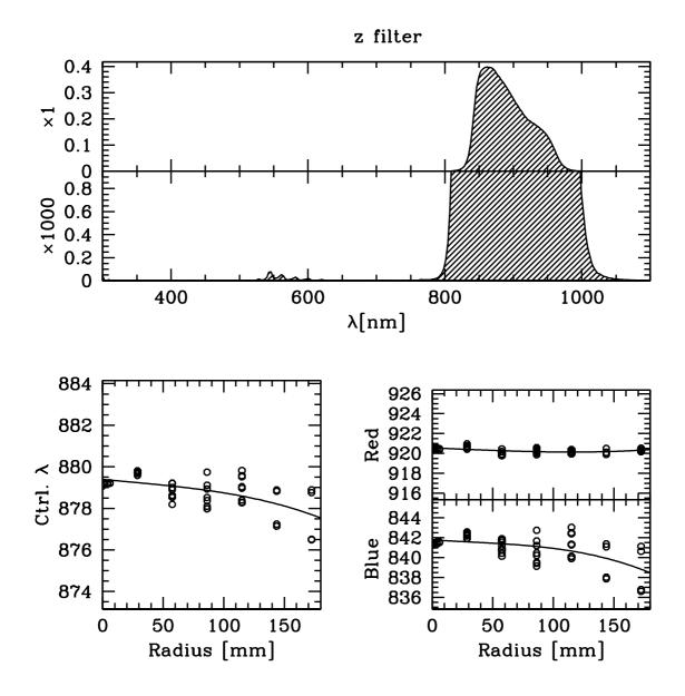
Figure 38: Top panels: throughput of the z' filter × average CCD response curve, including a blow-up by a factor of 1000 to show the out-of-band blocking. Bottom left: variation of central wavelength with radius on the focal plane (dots: measurements; line: polynomial fit). Bottom right: corresponding variation of wavelength at half-maximum throughput of the blue and red edges of the filters.
