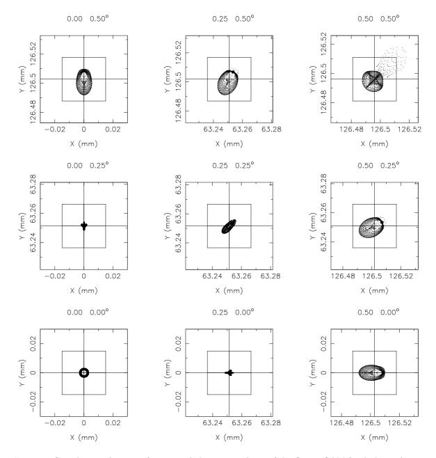
Figure 4: Sample spot diagrams for 500nm light in a quadrant of the OmegaCAM focal plane. A 2x2 pixel grid  $(30\mu m \times 30\mu m, \text{ corresponding to } 0.43'')$  is shown as well.
