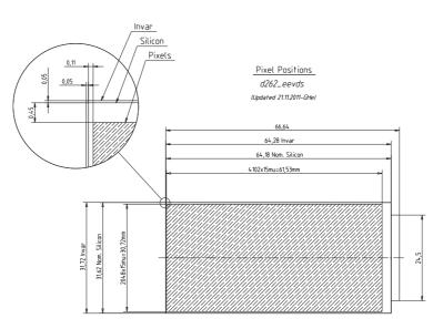
Figure 6: The light-sensitive area of a single CCD. Units are in mm, size of a single pixel is 15  $\mu$ .
