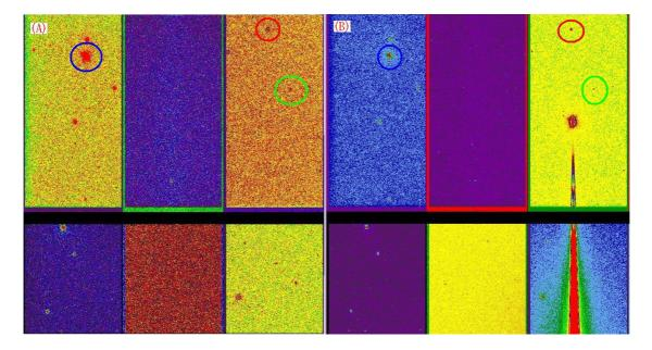
Figure 22: (A) A 300s exposure taken with the NB659 filter and OmegaCAM (B) A 20s exposure taken using the r\_SDSS filter on the same field. In both cases the PARLA laser was propogating (somewhat less powerful than the new 4LGSF system). Blue, red and green circles show stars visible on both images. The images are raw (no reduction has been performed). No laser light is visible when using the NB659 filter.
