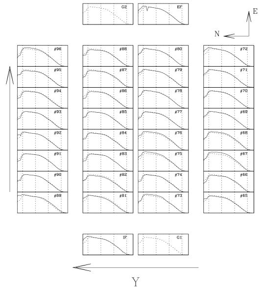
Figure 39: The QE curves for all CCDs in the mosaic, laid out as the mosaic itself (top view). The solid curve in each panel is the measured QE for that device; the dotted curve is the average for all 32 science CCDs. The wavelength range from 320 to 1100nm is plotted; dotted lines indicate 400, 600, 800 and 1000nm. X and Y are coordinates in the focal plane; for the default instrument rotator position angle of 0 X points East and Y points North.
