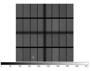
Figure 11: The shadow cast by the cross that separates the different segments of a composite filter (here the V filter).
