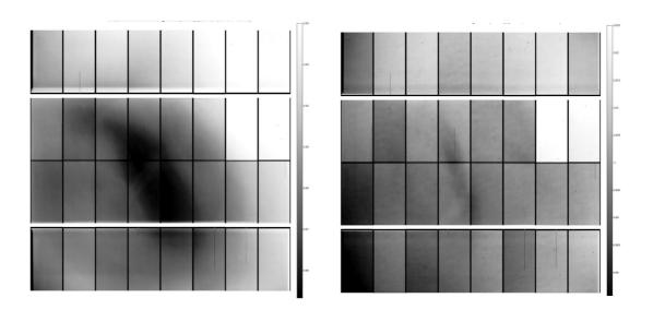
Figure 17: Raw r'-band dome flat divided by raw twilight flat taken at the same absolute rotator angles before and after the installation of the new baffling system (left and right panel, respectively).
