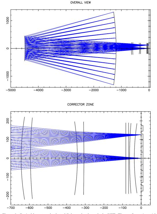
Figure 2: Optical layout and selected light paths through the VST. The configuration with the twolens corrector is shown. The bottom panel shows a zoom onto the corrector optics: the incoming light passes through two spherical lenses, a planar filter, and the spherical dewar entrance window before reaching the CCDs on the right. Scales are in mm.
