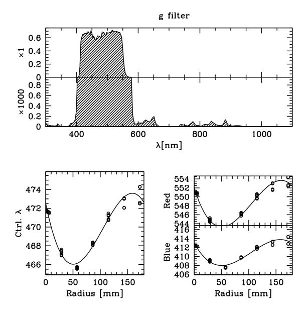
Figure 35: Top panels: throughput of the g' filter × average CCD response curve, including a blow-up by a factor of 1000 to show the out-of-band blocking. Bottom left: variation of central wavelength with radius on the focal plane (dots: measurements; line: polynomial fit). Bottom right: corresponding variation of wavelength at half-maximum throughput of the blue and red edges of the filters.
