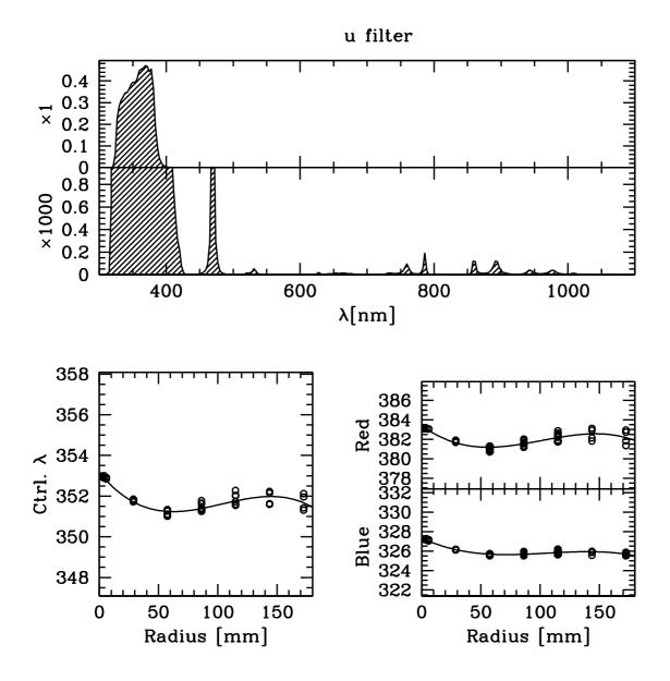
Figure 34: Top panels: throughput of the u' filter × average CCD response curve, including a blow-up by a factor of 1000 to show the out-of-band blocking. Bottom left: variation of central wavelength with radius on the focal plane (dots: measurements; line: polynomial fit). Bottom right: corresponding variation of wavelength at half-maximum throughput of the blue and red edges of the filters. The edge of the CCD array is reached at a radius of ~180mm.
