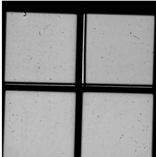
Figure 5-5: Flat field image of the SDI+ mode. The transmitted wavelengths are 1.6 mm (top left), 1.575 mm (top right) and 1.625 mm (bottom left and right).
