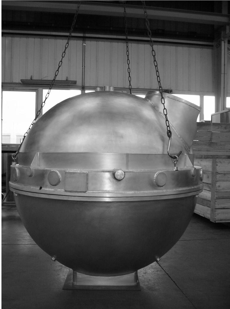
Fig. 5. The HAWK-I cold structure. The large reflective optics are mounted inside. One of the access hatches for filters and detectors is visible at top right.
