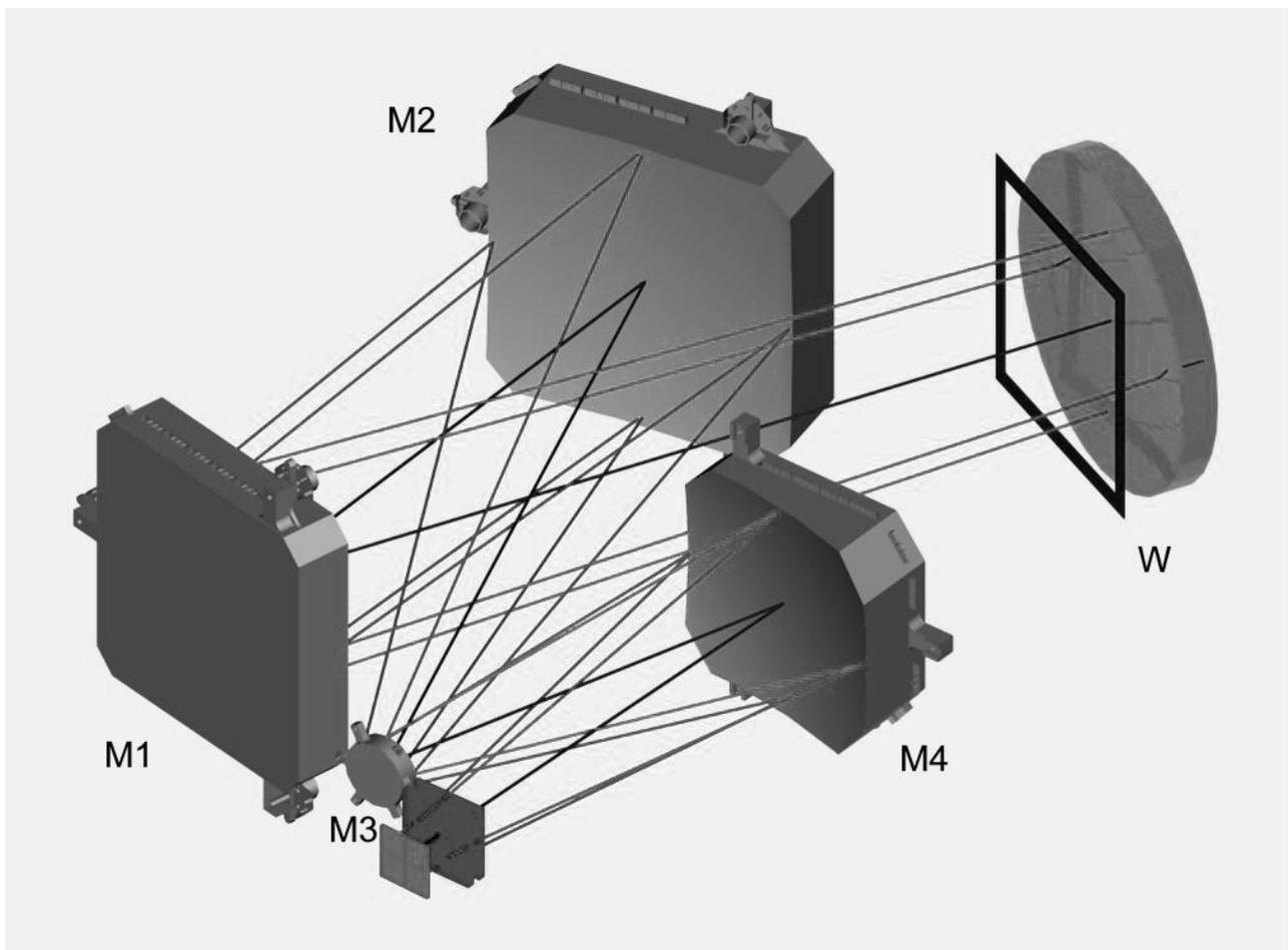
Fig.2 The HAWK-I optical layout. W is the cryostat window.
