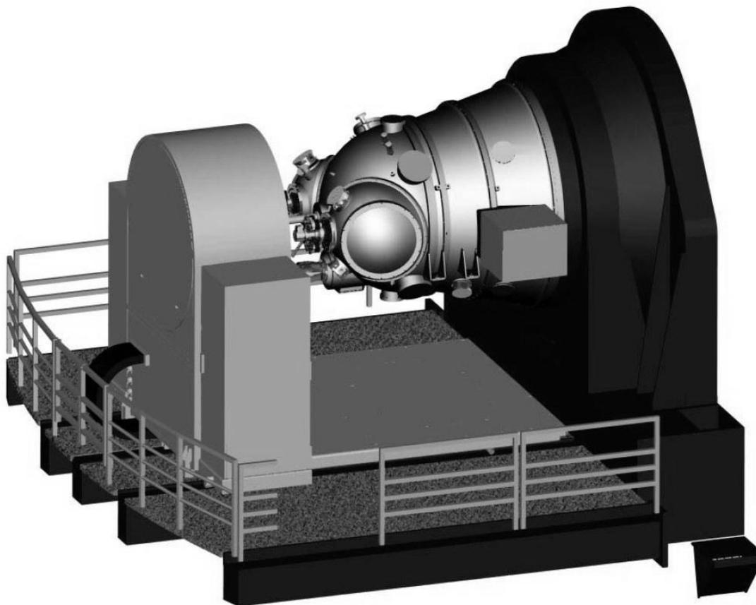
Fig. 4. HAWK-I shown mounted on the Nasmyth port of UT4. The large assembly to the left is the cable co-rotator. The HAWK-I space and mass budgets have margins to allow for the wavefront sensors and pickoffs required for the Adaptive Optics Facility (see section 6).
