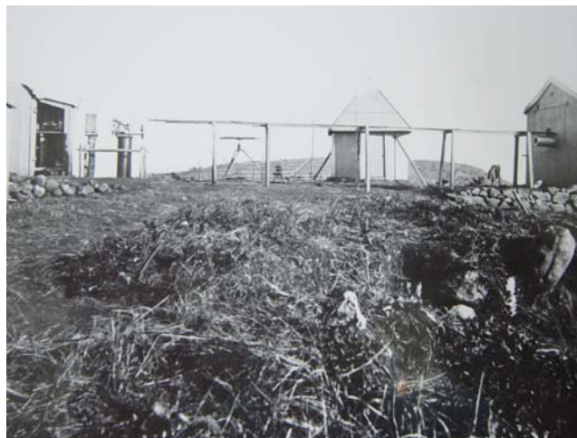
Figure 3: The setup of the U. S. Nagasaki station in 1874 with a photoheliograph (no photographs of the 1882 observing stations are available at U. S. N. O.): On the left side, a pillar carries the heliostat; the solar rays are deflected by a mirror and pass through a lens and a small tube into a hut (at right) where the photographic plates are exposed (U. S. Naval Observatory photograph; courtesy of Chuck Bueter).
