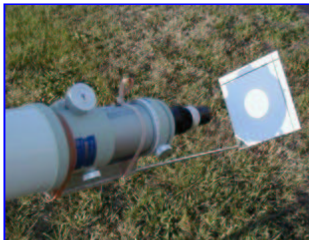
Image projection through the eyepiece
