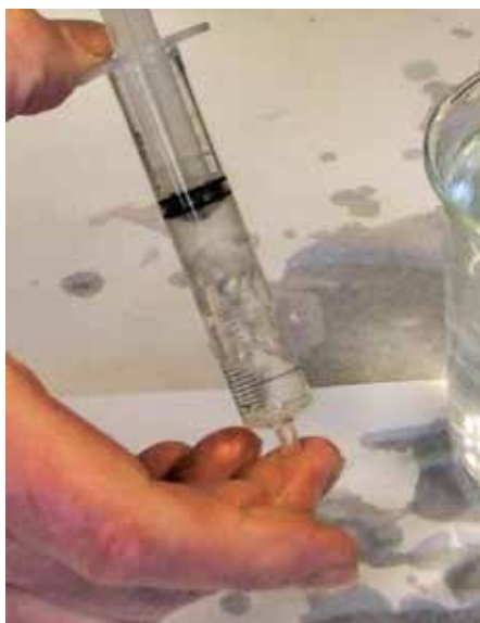
Figure 3: By creating a partial vacuum inside the syringe, students see how water boils when pressure is reduced.
