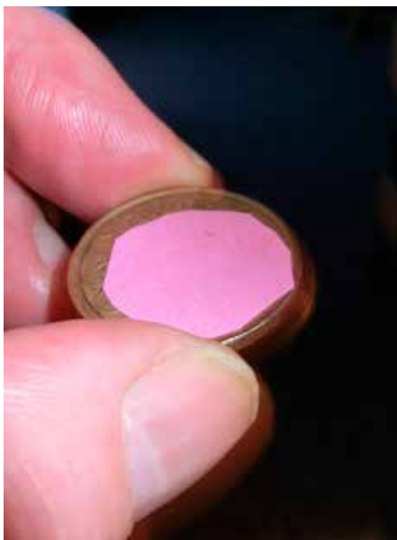
Figure 5: A piece of paper is placed on top of a coin, and the two objects are dropped together from a height to demonstrate air resistance.
