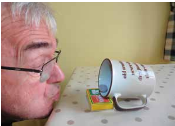
Figure 2: The coin is lifted into the cup by the reduction in air pressure above it.
