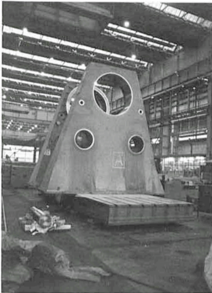
Figure 2: The fork arms on the reference plane. The seats (holes) for the drive units and for the big ball-bearing of the elevation axis are clearly visible.
