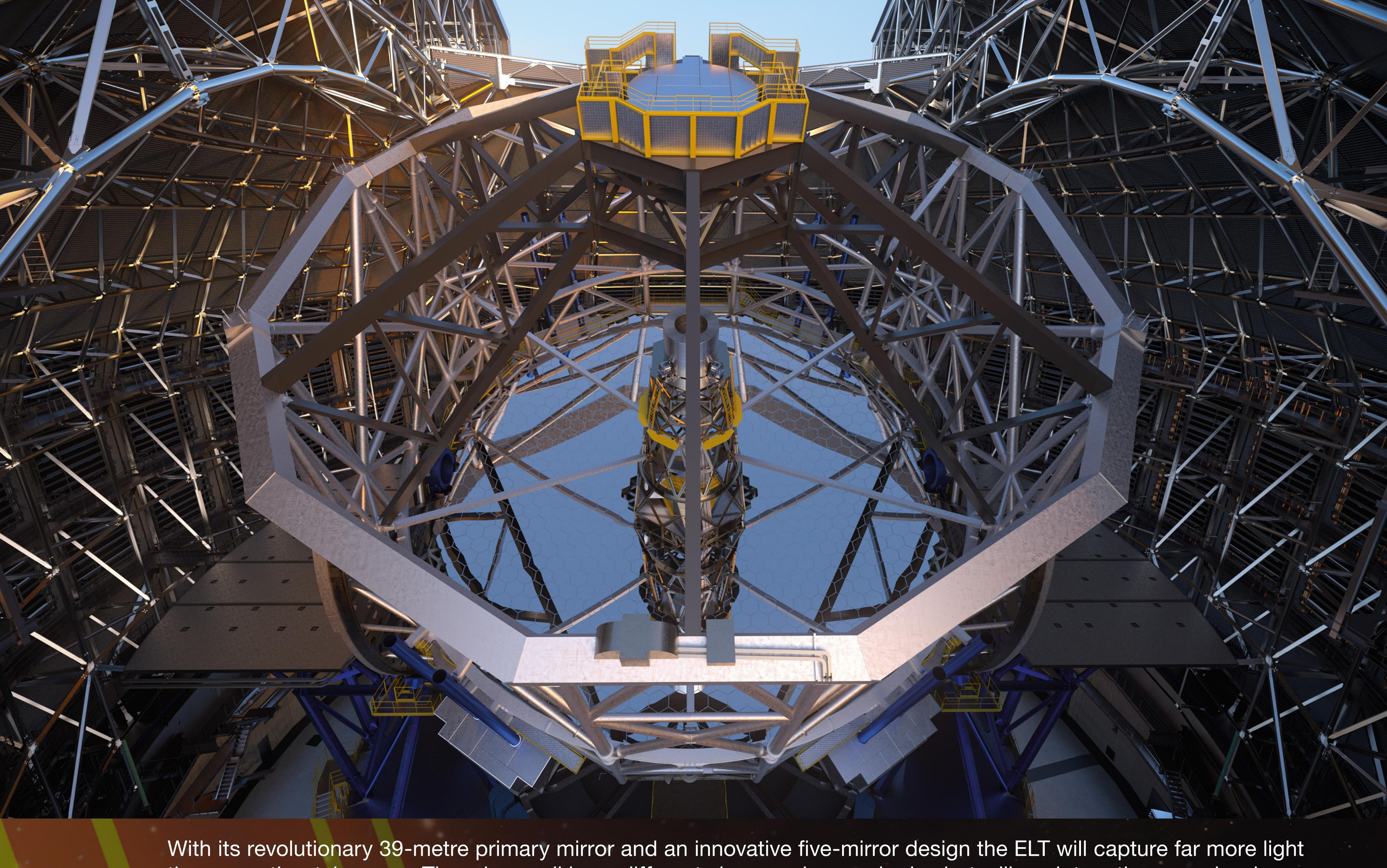
With its revolutionary 39-metre primary mirror and an innovative five-mirror design the ELT will capture far more light than any other telescope. The mirrors all have different shapes, sizes and roles but will work together seamlessly.
