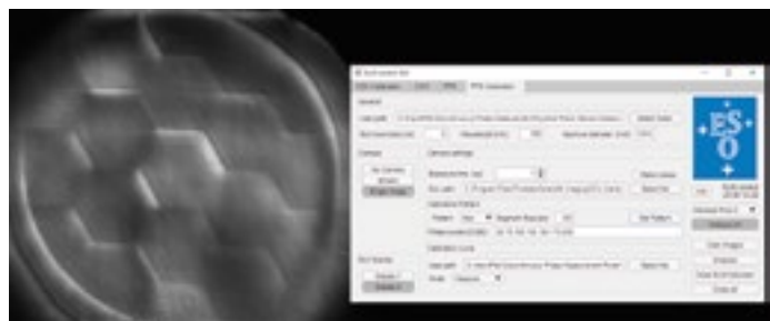
Emulating a segmented mirror using a spatial light modulator.
