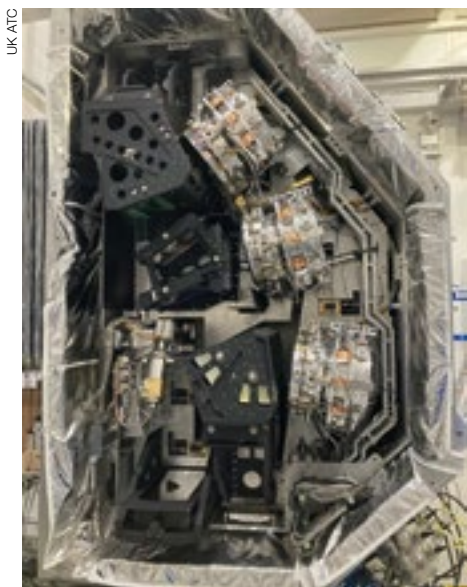
One half of the MOONS cryostat, showing three of the six cameras. The complete cryostat is 4.3 m tall and weighs 7.8 tonnes.
