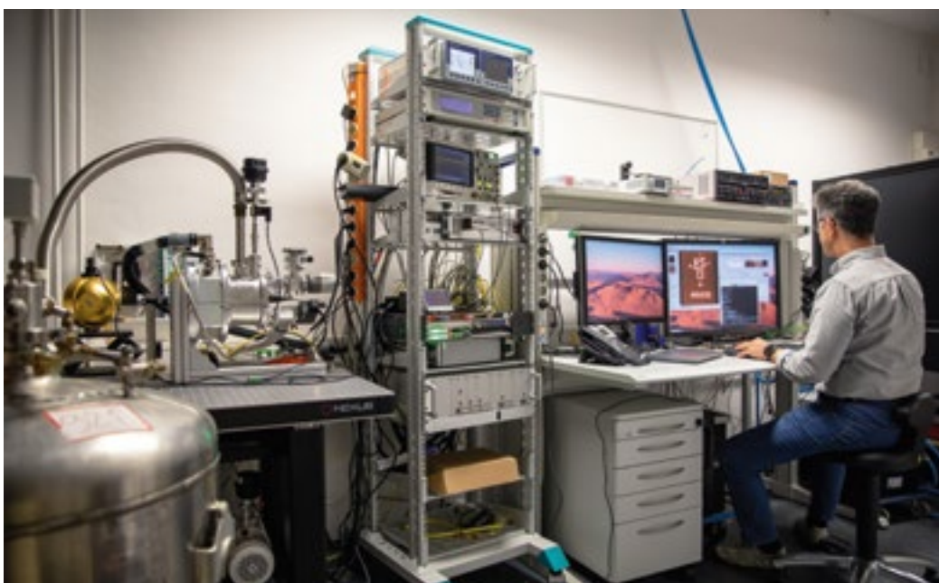
First light of NGCII in the laboratory, with a SAPHIRA infrared detector. From right to left: Leander Mehrgan, NGCII project leader, views the first light image of the ESO logo and the text NGCII; the detector controller (with green LEDs), in the electronics rack; the system used to project the ESO logo, on the optical bench; and the detector cryostat.
