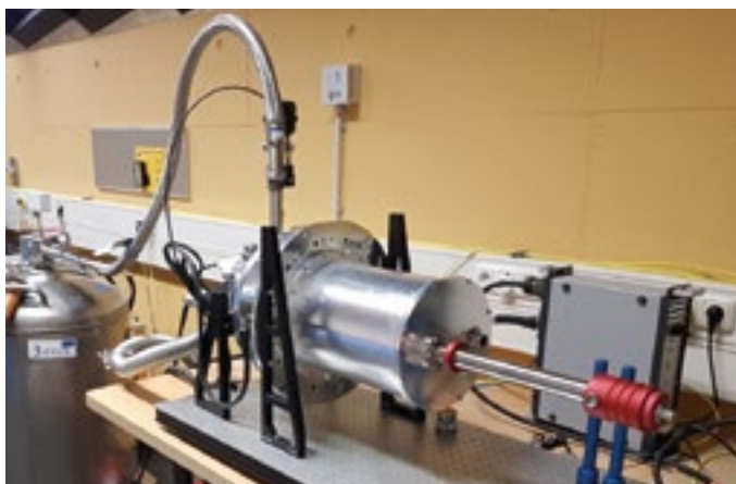
CCD qualification setup with iron-55 source.
