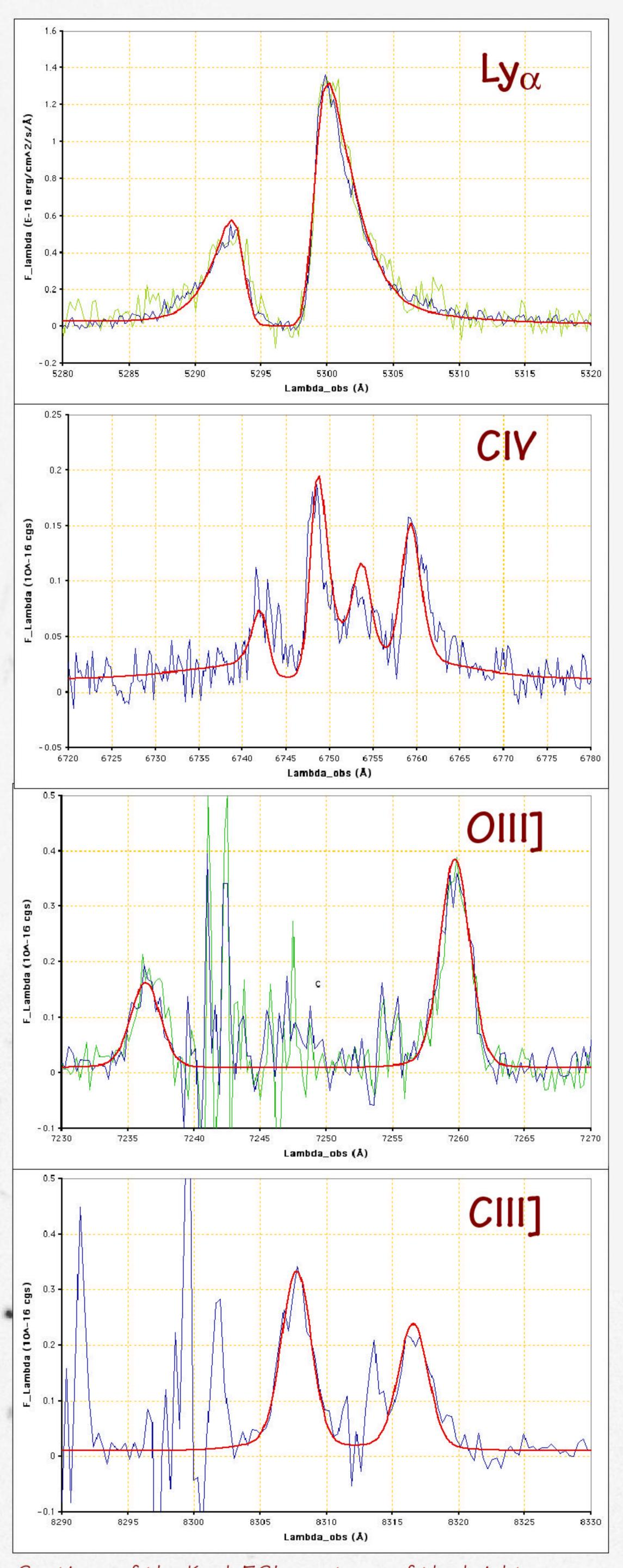
Sections of the Keck ESI spectrum of the brighter arc component plotted as observed flux per unit wavelength vs. observed wavelength. Regions which appear in two orders appear as overplotted spectra. The red lines show gaussian fits from which the velocity dispersions and line strengths are derived. Both  $Ly_{\alpha}$  and CIV include absorption components with pure gaussian absorption coefficients.
