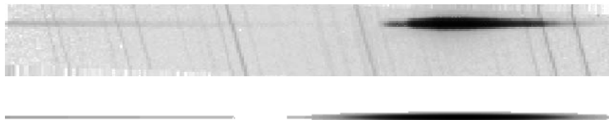
Figure 3. Na layer plume (right side) and Rayleigh cone top (just seen at the left side) as seen from the 2.2 m telescope (top) and as modeled (bottom). The image size is 600 \times 80 \text{ arcsec}^2 . Images are in linear scale
