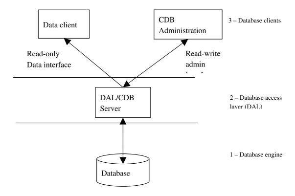
Data clients can be Components (that read the CDB) as well as tools like the cdbBrowser. Data clients can also write the CDB, changing the actual content of the database, through an administrative interface. The cdbBrowser utility can also be used to edit the database.
