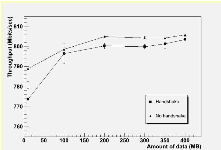
Figure 6: Performance comparison between hand-shake and no hand-shake mechanism; note that with increasing amount of data, the overhead due to the hand-shake mechanism decreases.
