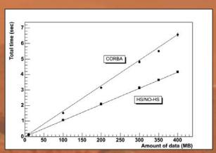
The figures above represent the results of our performance tests. The throughput, i.e., the number of bits per second, vs different amounts of transmitted data is shown on the left and middle pictures. It clearly appears that the ACS Bulk Data mechanism is always better than using simple CORBA call (the estimated gain is around 30%) and that the hand-shake mechanism does not introduce relevant performance penalties respect to the no hand-shake case.
