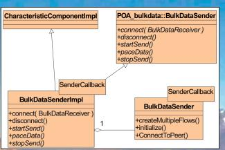
The ACS Characteristic Component relative to the Sender is implemented as a C++ template class. The template parameter is a callback which can be used for sending asynchronous data. This callback provides methods for sending data at predetermined user-configurable time intervals. To allow sending data in a synchronous way, a default callback is provided, which disables the asynchronous mechanism.
