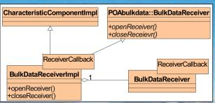
The ACS Characteristic Component relative to the Receiver is implemented also as a template class. The template parameter in this case is a callback, which has to be provided by the user
