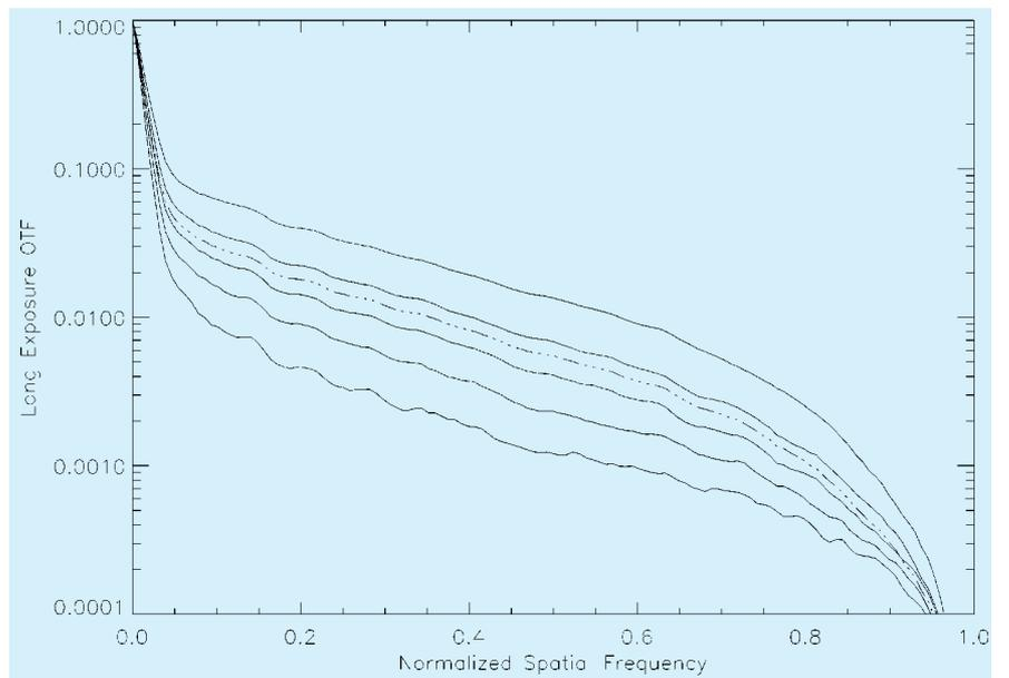
Figure 2: The OTFs are estimated for the following seeing values: from top to bottom,  $0.65$ ,  $0.73$ ,  $0.79$ ,  $0.85$  and  $0.93 \text{ arcsec}$ . The corresponding SRs are respectively:  $3.8\%$ ,  $2.1\%$ ,  $1.3\%$ ,  $0.8\%$  and  $0.4\%$ . The mean OTF is also drawn (dashed line).
