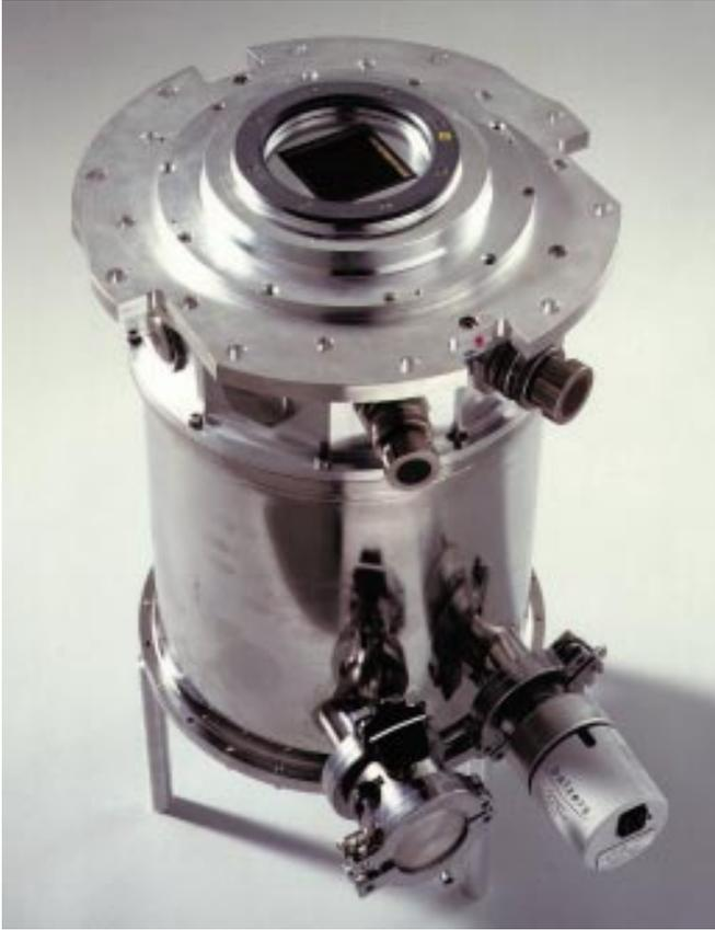
Figure 2 : Bath cryostat, Cassegrain version.
