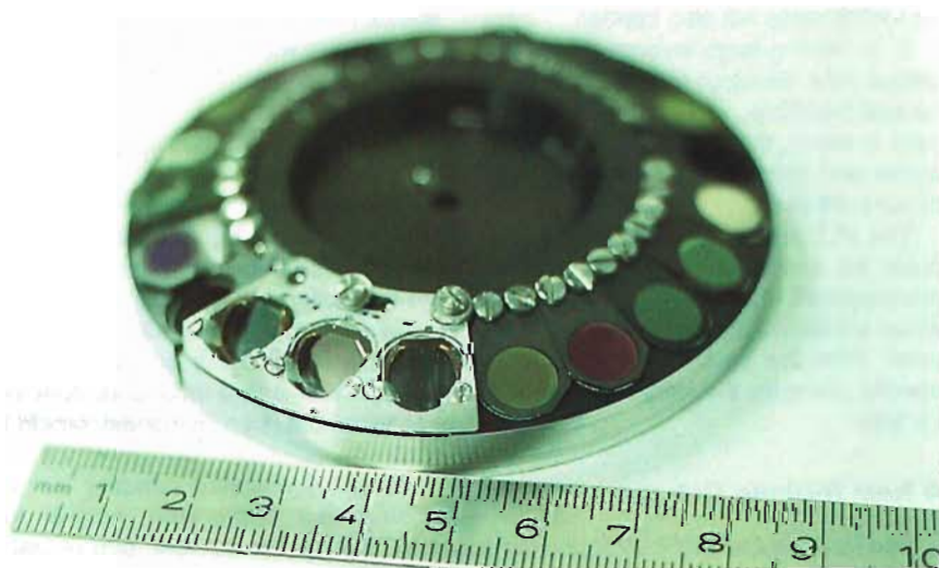
Figure 1: The rare but essential ingredients are shown. The three grisms are mounted in one fixture to the filter wheel. For each grism the order sorting filter, the base prism and the silicon wafer carrying the diffractive structure had to be mounted in a space of less than 1\ \text{cm}^3 . The mount needed to be designed compatible with operation at 60 K. The silicon wafer is mounted in direct optical contact to the prism, and great care was required during assembly to avoid contamination of the optical surfaces. It was also required to carefully adjust the orientation of the grooves parallel to the apex of the prism.
