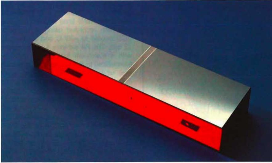
Figure 1: Photograph of the R4 prototype. The dimensions are 450×130×70 mm; the dead space between the two segments is 14 mm wide.
