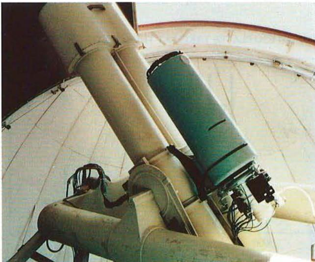
Figure 3: The 40-cm reflector mounted on the GPO at La Silla.
