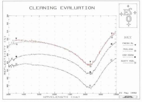
Figure 2: Comparison of cleaning techniques.
