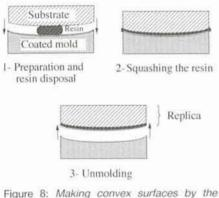
replica technique. Prior to making the replica, the mould is coated with a reflecting substrate which at the end covers the external resin surface. The final thickness of the resin layer is 50  $\mu$  (from P. Assus, O.C.A.).
