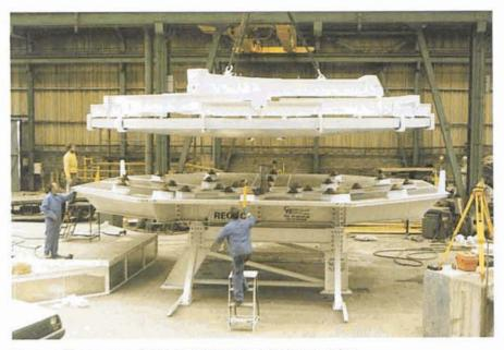
Figure 1: Dummy mirror being loaded onto the transport container.
