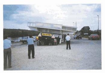
Figure 3: "Rock-and-roll" test on the hydraulic platform.
