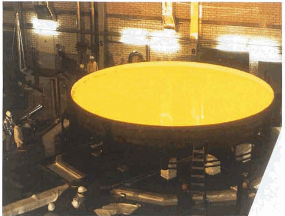
The first 8.6-m mirror blank at Schott, shortly after the molten glass was poured into the rotating form (Photo: Schott).
