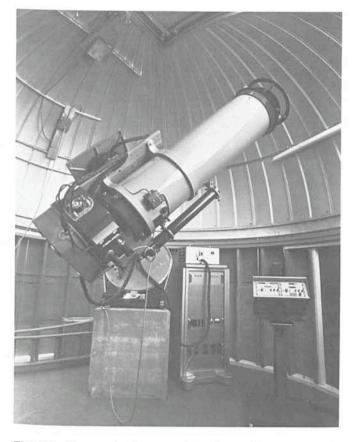
The 40 cm Cassegrain telescope of the Geneva Observatory on La Silla. The photoelectric photometer is at the Cassegrain focus.
