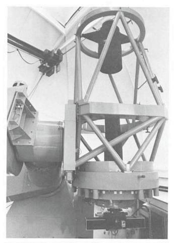
Fig. 1: CORAVEL mounted at the Cassegrain focus of the 1.54 m Danish telescope at La Silla.
