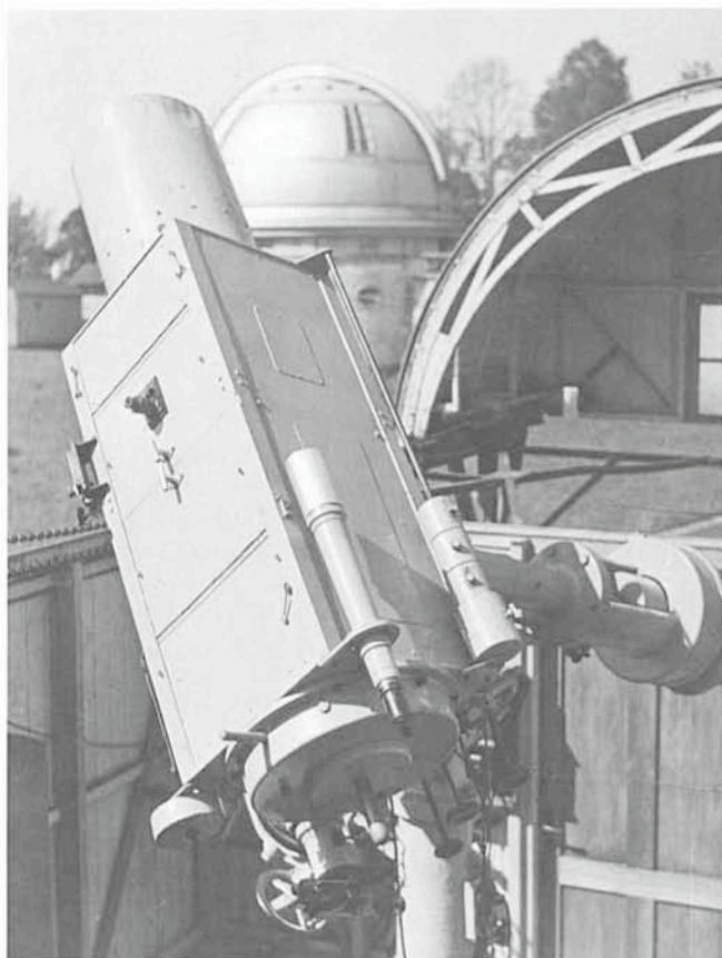
Fig. 2: The Original Schmidt Telescope at the Hamburg Observatory;  $f/1.75$ ,  $15^\circ$  field.
