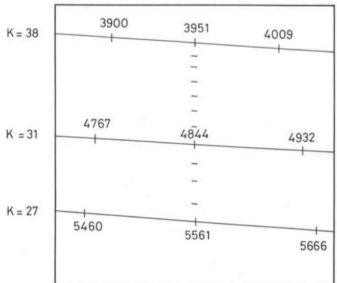
Fig. 3: Schematic of an echelle spectrum.  $K$  is the echelle grating order. Wavelengths are shown in Angstroms. Intermediate orders are shown by tick marks. The circumscribed square is the 25 mm  $\times$  25 mm target area of the SEC Vidicon.
