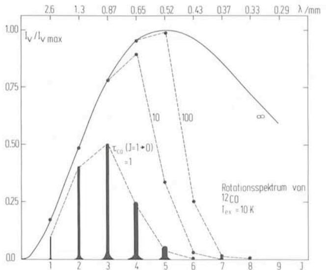
Fig. 3: Intensities of rotational lines  $J \rightarrow (J-1)$  of the  $^{12}\text{CO}$  molecule computed by Schmid-Burgk for a plane-parallel gas layer in TE at  $10 \text{ K}$ . Curve parameter  $\tau_{\text{CO}} (J=1 \rightarrow 0)$  is the optical depth for the lowest rotational transition. The curve  $\tau_{\text{CO}} \rightarrow \infty$  corresponds to the Planck curve. Note that the width of rotational lines increases approximately proportional with  $J$ .
