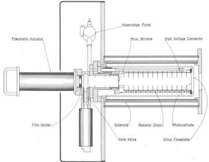
Fig. 1: The RGO 4 cm electronographic camera (schematically).
