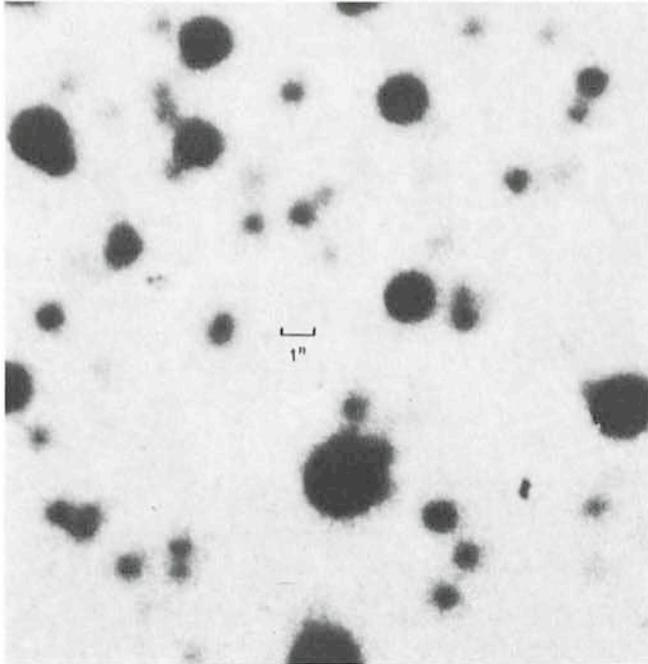
Fig. 1: Enlargement from a 1-hour exposure on IIIa-J emulsion behind a GG385 filter, showing stars in the globular cluster NGC 3201. The images are perfectly round and measure about 0.5 arcsecond in diameter. Danish 1.5 m telescope; observer Dr. B. Niss, March 7, 1979. Average zenith distance 18°.
