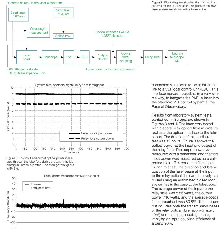
The infrared laser wavelength was also measured and logged during the test and Figure 4 shows the measured frequency error, in MHz, from the nominal set point during the test. The deviation is within a few MHz, which meets the goal
