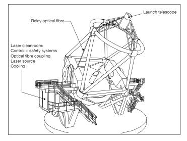
Figure 1. Sketch of VLT UT4 showing the main parts of the Laser Guide Star Facility.
