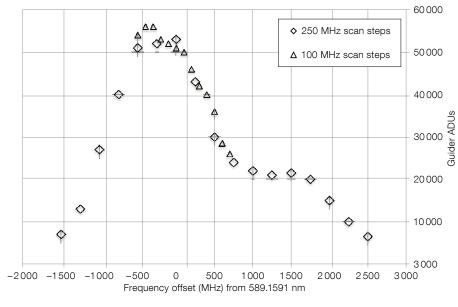
Figure 6. A wavelength scan through the sodium  ${\rm D}_{\rm 2}$  doublet taken during commissioning.
