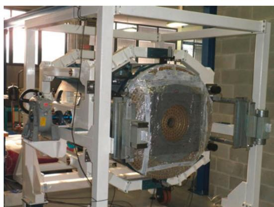
Figure 2. Finite element modelling of the complete DSM shown on the left. It is used as a baseline to compare with the experimental results. On the right, the hub with dummy weights and external encoders to measure flexure. The hub integration and service stand allows the inclination of the hub to be varied to characterise the flexure at the level of the reference body for different orientations. The results of the flexure campaign confirmed the system rigidity at  $150\ \text{N/mm}$ .
