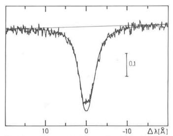
Fig. 2: Intensity tracing of  $H\gamma$  (superposition of three plates). The smooth curve is the computed profile of the final non-LTE model. In the line core the observed profile is filled up by the emission of the Carina nebula around HD 93250.
