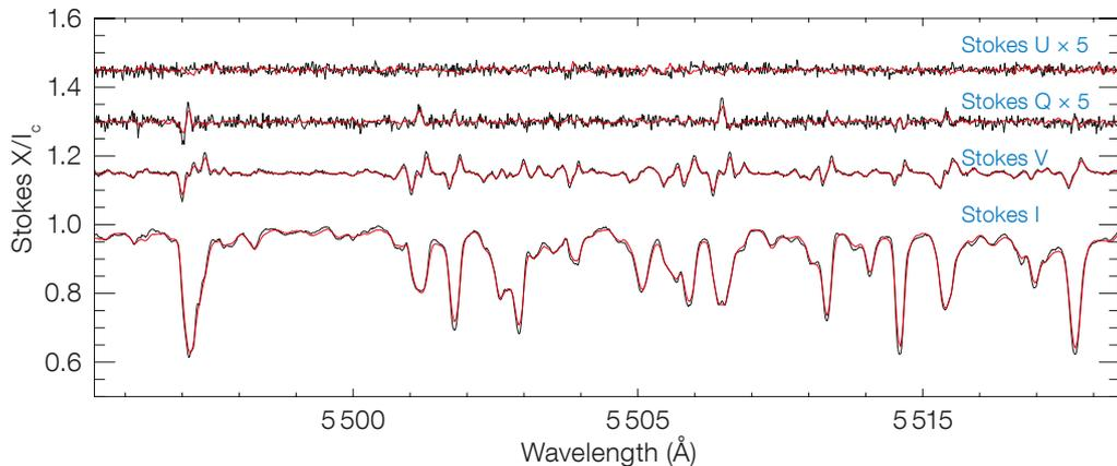
Figure 5. Comparison of the Stokes spectra of a standard magnetic star  $\gamma$  Equ taken at the CFHT with the ESPADONS spectropolarimeter (red line) and with HARPSpol (black line) is shown. The ESPADONS spectra were taken as part of CFHT's calibration and engineering plan, and were retrieved from the Canadian Astronomy Data Centre. The visible differences are mostly due to the higher resolving power of HARPS.
