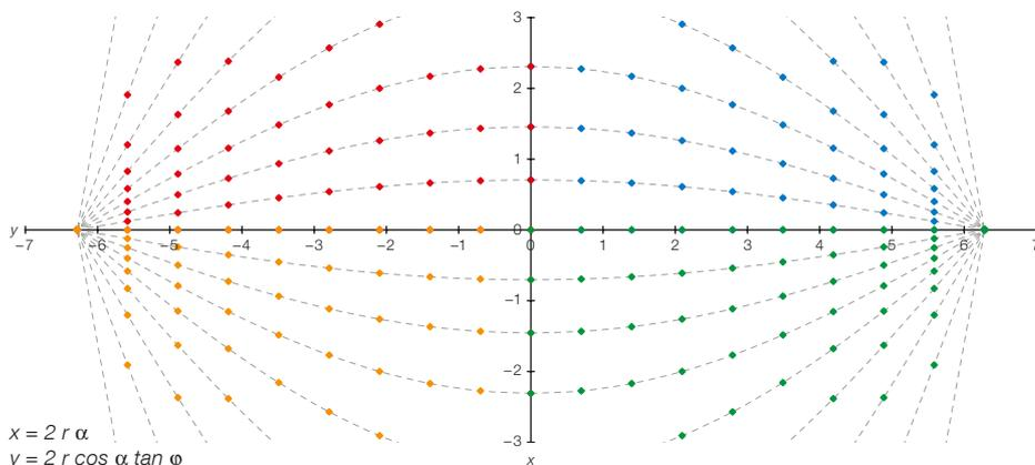
Figure 9. A representation of the projection of altitude and azimuth in a cylindrical pinhole camera is shown. The coloured points are separated by 10 degrees and the  $x$  and  $y$  scales are in units of cm for the solargraph cans used here.  $x$  and  $y$  are the horizontal and vertical coordinates,  $r$  is the radius of the can, and  $\phi$  and  $\alpha$  are the altitude and azimuth angles respectively.
