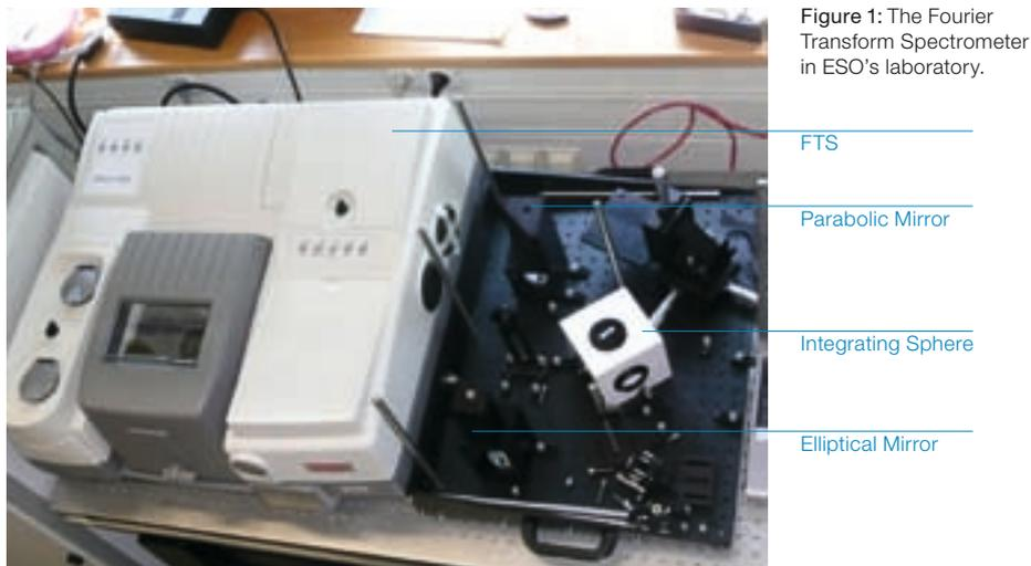
Figure 1: The Fourier Transform Spectrometer in ESO's laboratory.
