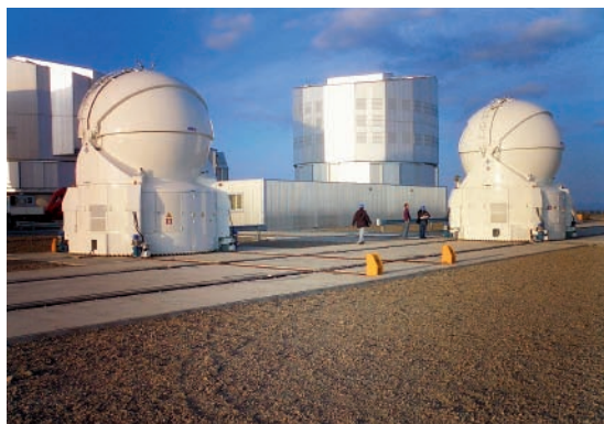
Figure 3: A recent photograph taken on the VLTI platform in January 2005 by Bertrand Koehler. The first two ATs, located at station E0 and beside G0, are shown in the foreground, as well as UTs 3 and 4 (MELIPAL and YEPUN) in the background. The building that can be seen in between the ATs is located on top of the interferometric lab, where the beams coming from the UTs or ATs are combined. The beams are sent through an underground light-duct system to the interferometric lab. Courtesy B. Koehler.
