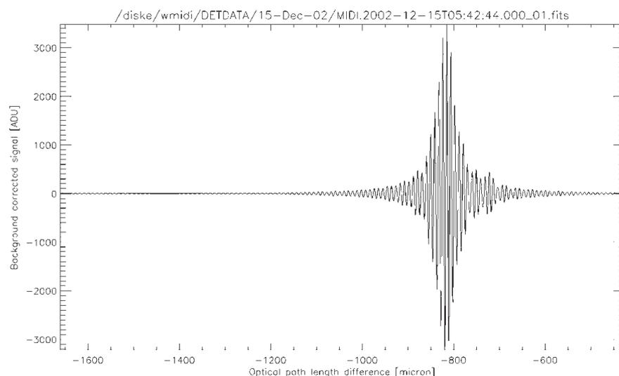
The upper image shows the “first fringes” of the star Epsilon Carinae, as obtained at VLTI with the new MIDI instrument at the mid-infrared wavelength of 8.7  $\mu\text{m}$ .
