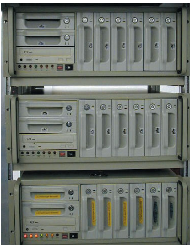
Figure 2: This figure shows three of the NGAS units mounted in a rack. They are fully equipped with eight disks each, giving a total of 1.65 terabyte of on-line storage capacity with three processors running at 1.2 GHz each.
