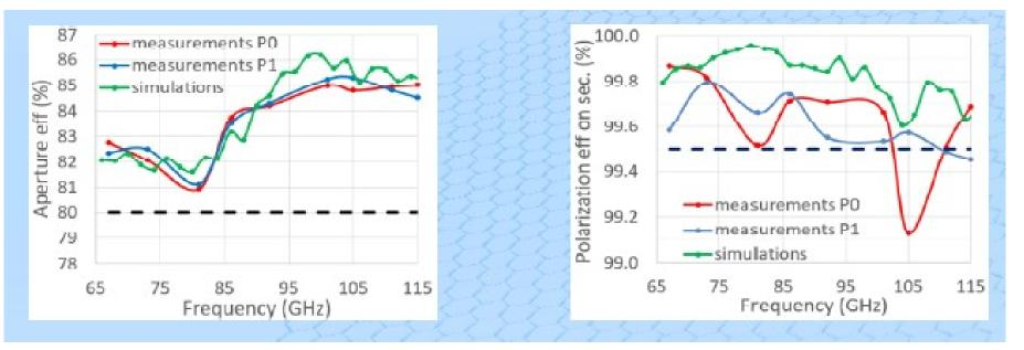
Phase A Band 2+3 optics tests at ESO
