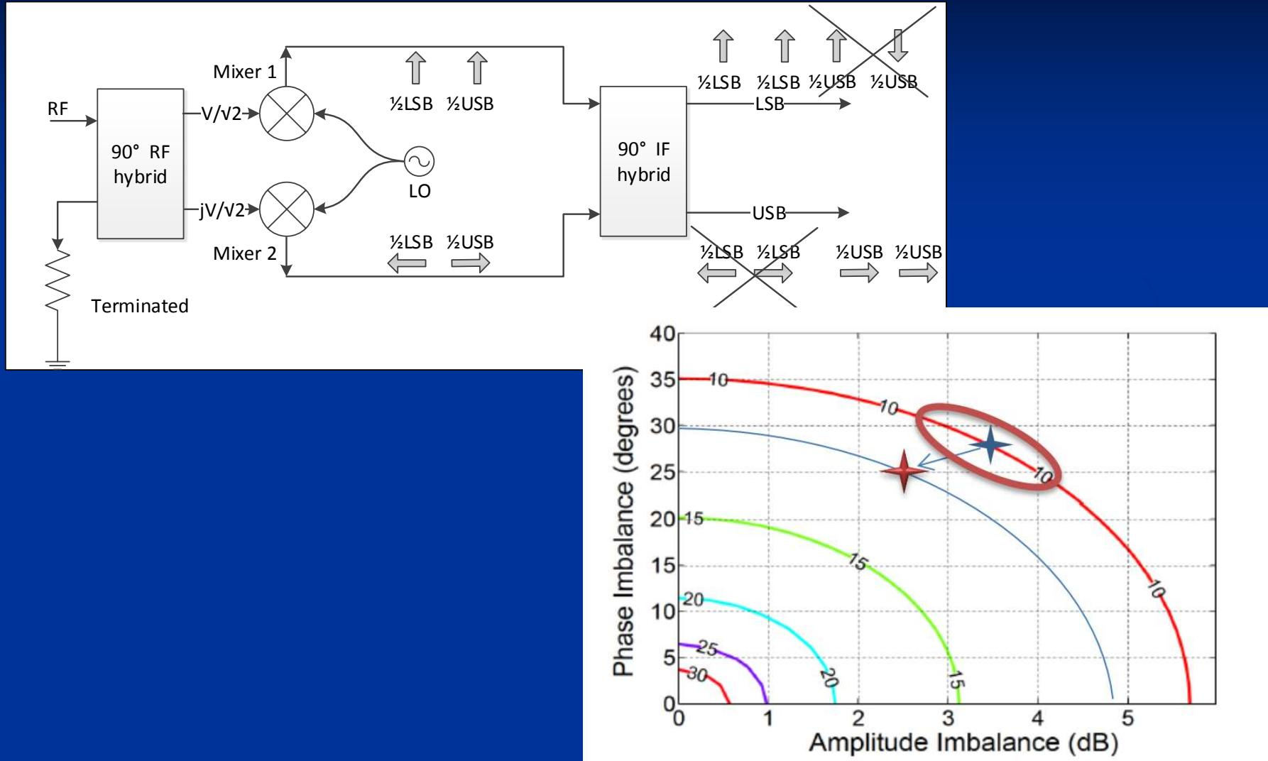
15  $\mu\text{m}$  substrate offset gives 12.5 degree in phase;
