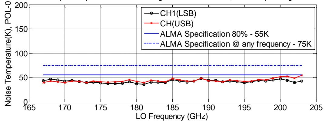
True (Corrected for sideband rejection) Average Noise Temperature measured over, IF = 4 GHz - 8 GHz
