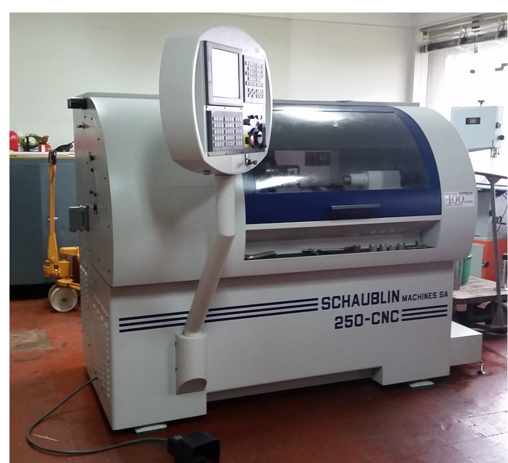
Fig. 1. High-precision ( \sim 1 \mu\text{m} ) CNC milling machine and lathe.
