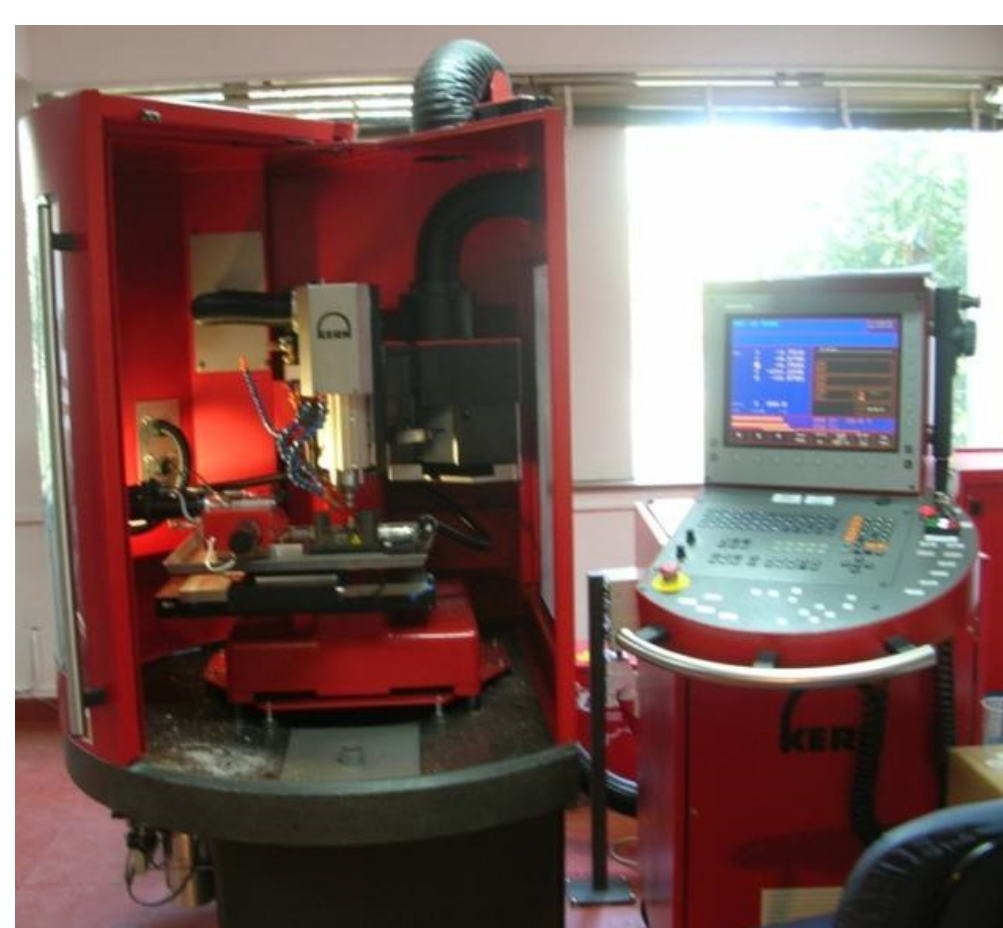
Fig. 1. High-precision ( \sim 1 \mu\text{m} ) CNC milling machine and lathe.
