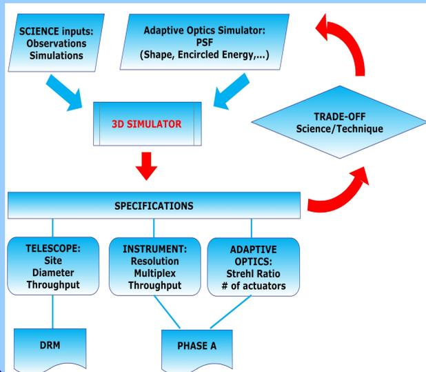
The end-to-end simulator produces datacubes in FITS format, mimicking the result of real observations. An AO system can be modeled through its PSF, which is simulated using a dedicated pipeline (e.g., Neichel+08, JOSAA, 26, 219)
