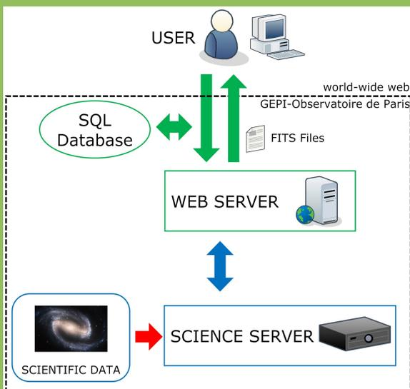
The user interface (see web forms on the top-right) is hosted on a secured served called **WEBSIM**. The simulations are run on a science server. When completed, an email alert is sent and the products (FITS files) can be downloaded.
