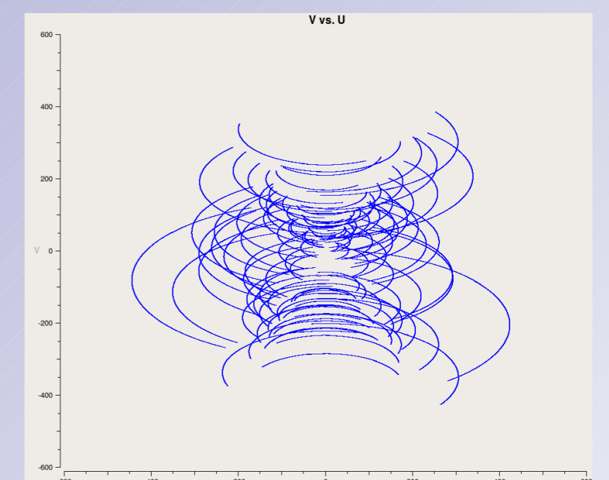
Simulated uv -coverage for an 8-h observation
